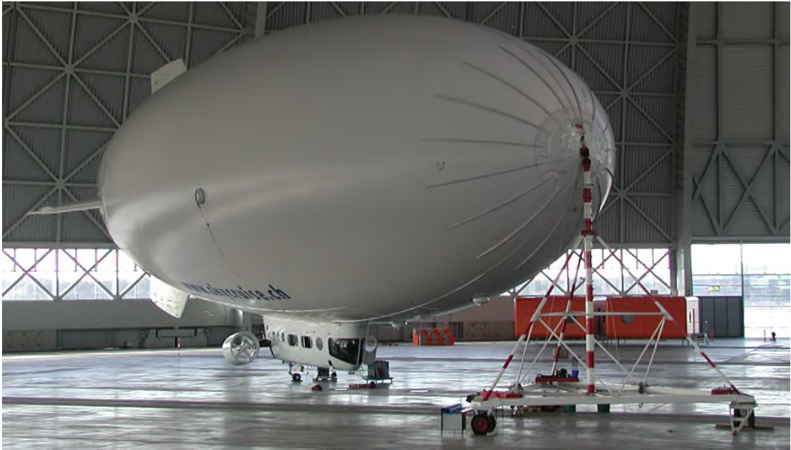
Tripod Mast for manoeuvring Skyship in the hangar
